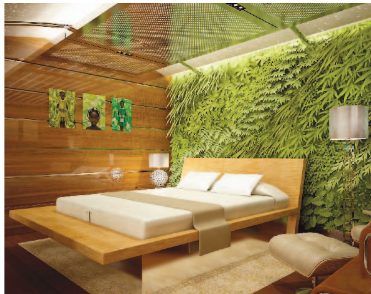
Edese Doret's Boeing 787-9 interior design features living walls made of ferns. The walls include an irrigation system to carry both water and food to the plants.
